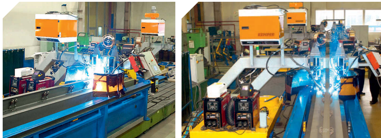
ROBOTIC CENTER FOR CENTER SILL LONGITUDINAL SEAM WELDING
