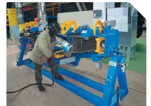
Front beams assembly stand
