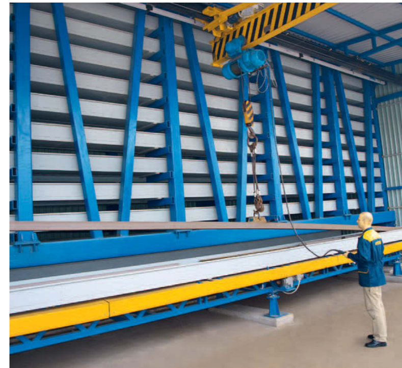
Automated storage system for section material
