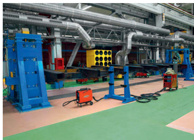
Rotator with vertical lift, load carrying capacity 10 t
