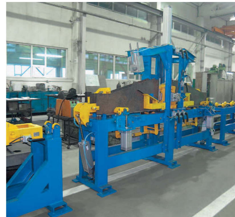
Bolsters assembly and welding line
