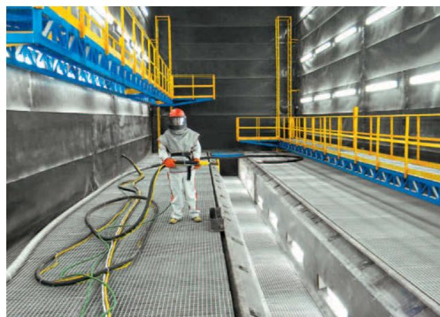
Shotblasting chamber for cars
