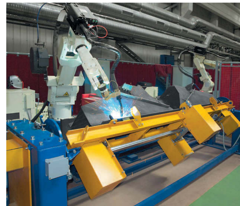
Gondola car underframes assembly and welding stand
