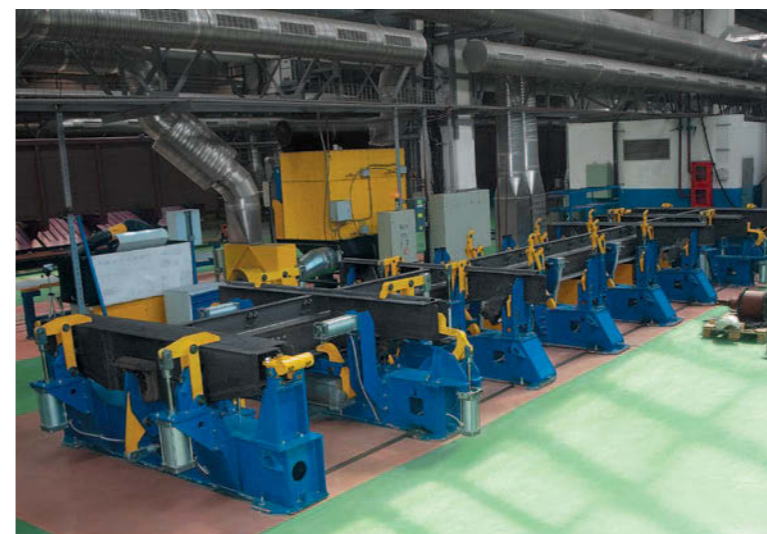
Gondola car underframes assembly and welding stand
