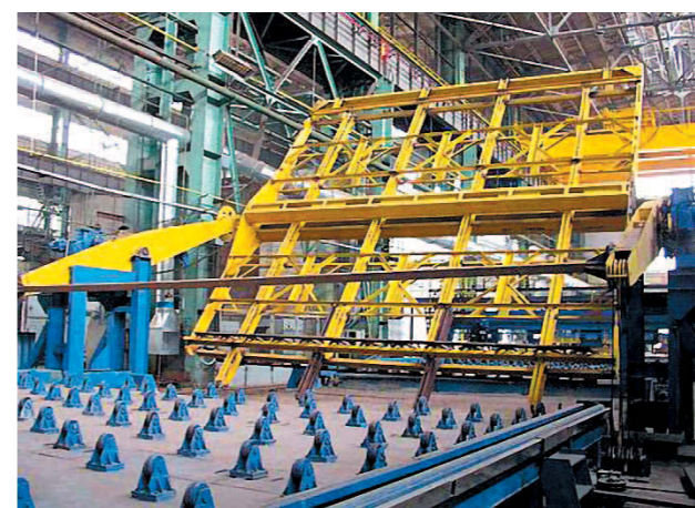
Sheet assembly and welding line
