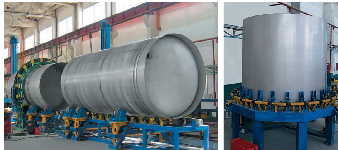
Tank assembly and welding line
