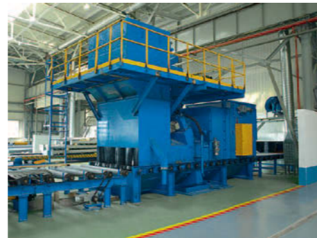
Shotblasting chamber for cleaning of metal-roll
