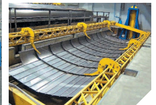
Rotator for roof welding
