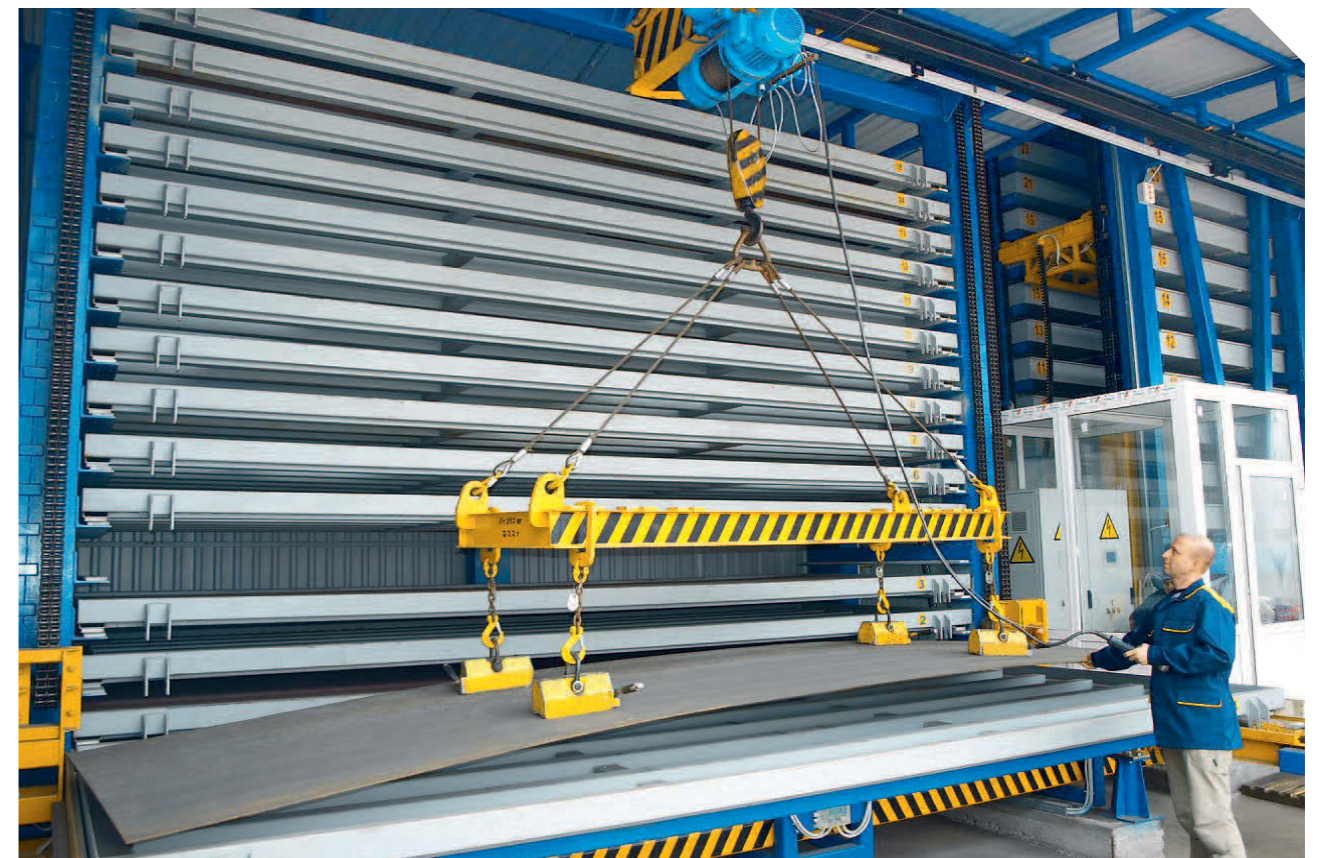
Automated storage system for sheet products
