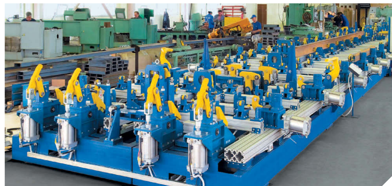
Multipurpose jig for assembly and welding of passenger car underframes
