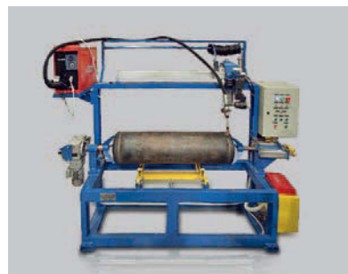
Stand for automatic head-to-shell welding
