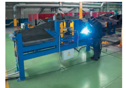
Intermediate beams assembly and welding line
