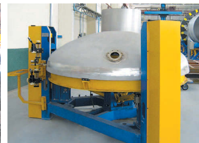
Tank head assembly and welding, edges trimming stand
